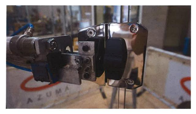
Figure 2: Tested Latch
